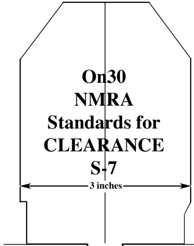
Figure 3, NMRA Clearance Gauge (Full Size)
